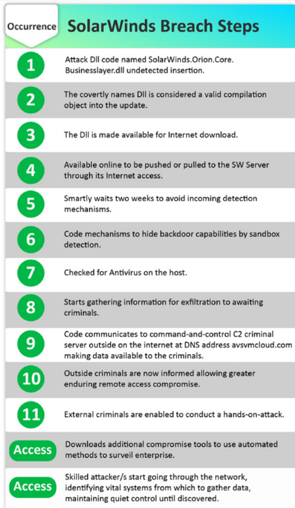
Fig 1 Diagram Depicting Eleven Breach Steps
